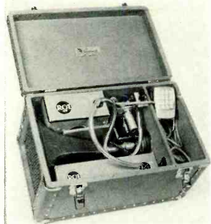
A top view of the PA system with the cover open to show major components.
